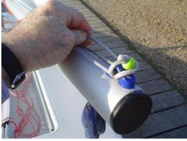
b. Make a loop through the boom end fitting
