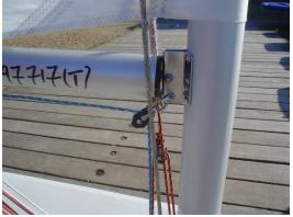
b. The line then returns under the boom on the other side and is tied off into the loop in the Elastic.
